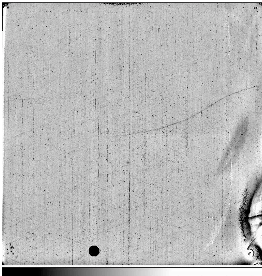
Figure 4: The resulting normalised flat-field image for the G102 grism at 10000\text{\AA} , derived from the image shown in Figure 3. The greyscale is \pm 20\% about the mean.
