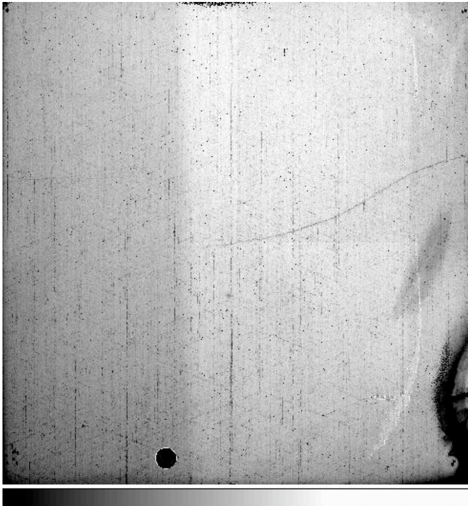
Figure 3: Example of the monochromatic image at 10000\text{\AA} taken with the G102 grism. The mean level is 12330 ADU and the greyscale range \pm 20\% about the mean (black - white).
